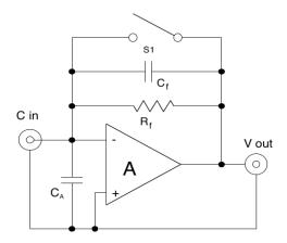
Figure 2: THE CHARGE AMPLIFIER (SIMPLIFIED SCHEMATIC)
