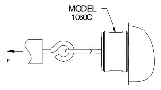
PROPER TENSILE LOADING USING THREADED HOOK EYES
