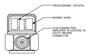
Figure 1-Cross section, series 3055D
