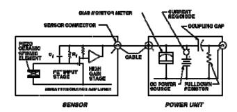
Figure 2-Electro-mechanical schematic, accelerometer and power unit system.
