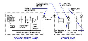
Figure 1-Electro-mechanical schematic, accelerometer and power unit system.
